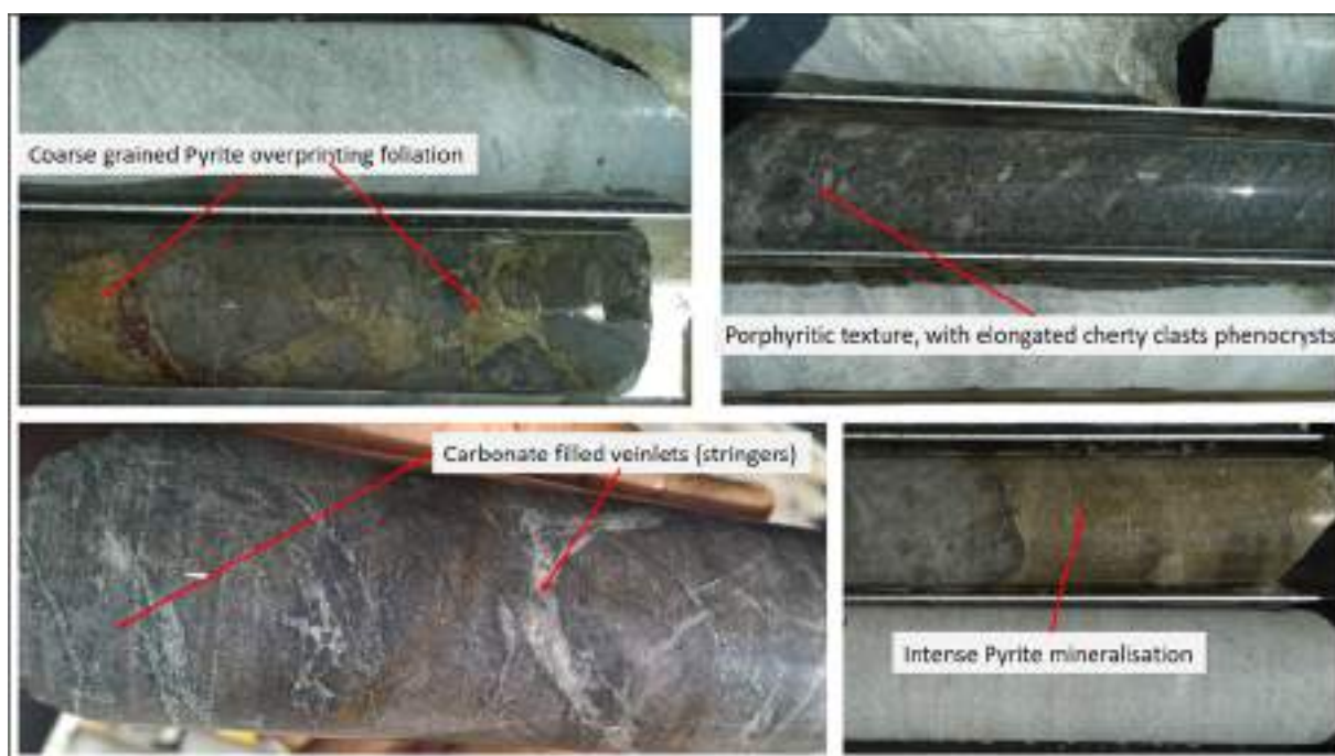
Photo 1: Photo showing metasediments with carbonate filled veinlets, porphyritic texture and coarse-grained pyrite from Surface Exploration Drilling core.
