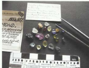
Heavy mineral concentrate (Total weight 4.974g) from the Somabula alluvial deposit. One diamond crystal (octahedron/dodecahedron) of gem quality (0.145g) is featured in the centre. Other gems shown are: chrysoberyl, alexandrite, sapphires, garnet, amethyst, topaz ("Somabula blue" and white), aquamarine, hoari and native gold.
