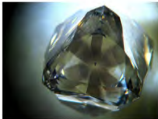
An octahedral crystal (7.38mm apex to apex), with one re-polished face, shows a six-ray star phenomenon. A few tubular inclusions and one small octahedral diamond inclusion at the centre are also evident. Photograph by Grant Pearson (2014)
