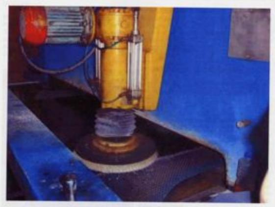
The time for polishing depends on the size of the slab and also on whether the slab is fine or coarse. Thus, the slabs are polished on one side until they are shirty! After the polishing process, the slabs are packed in the warehouse for export. The company sells their products to South Africa, Brazil, Argentina, America, England, Israel, Australia, Bulgaria and Italy. The major costs of the company are the steel grits, electricity and the blades.
