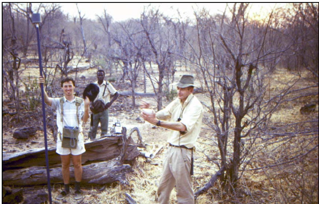
Figure 8. The September 1994 Sinamwenda Expedition team doing a ground magnetometer traverse. Left to right: Dr Kevin Walsh (holding a proton-precession magnetometer), Game-Scout Kamin (holding a rifle), and Dr David Robertson (holding a GPS). Photograph by Sharad Master.
