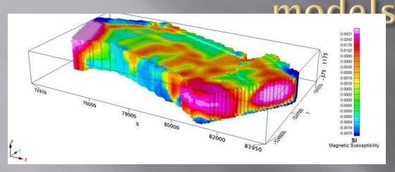
The final 2.5D model for each line was exported in Mag2dc as an ASCII file. The algorithm 'Magmodintrp' written in FORTRAN 77 by Prof Edgar Stettler was then used to extract the cross sections of the final model giving an X, Y, Z file.
