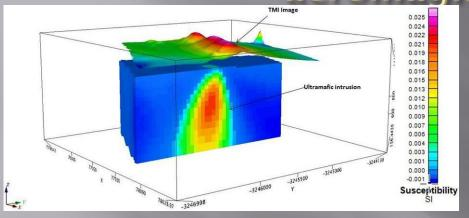
Voxel inversion, by definition, divides the earth into a number of voxel (cubic) elements and solves for their associated physical properties (magnetic susceptibility in this case).
