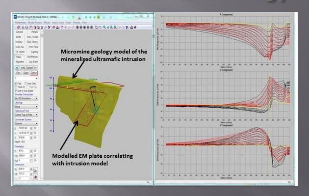
Modelling results for borehole JMP002 showing the modelled EM plate integrated with the Micromine geology model of the mineralised ultramafic intrusion. The right hand window shows the measured EM response profiles in black and the modelled EM response in red for the three components A, U and V.
