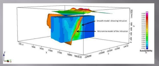
• However the slightly magnetic material south of the sill which has been resolved by the Mag2dc inversion process shown on the right does not appear on the VOXI inversion results.
