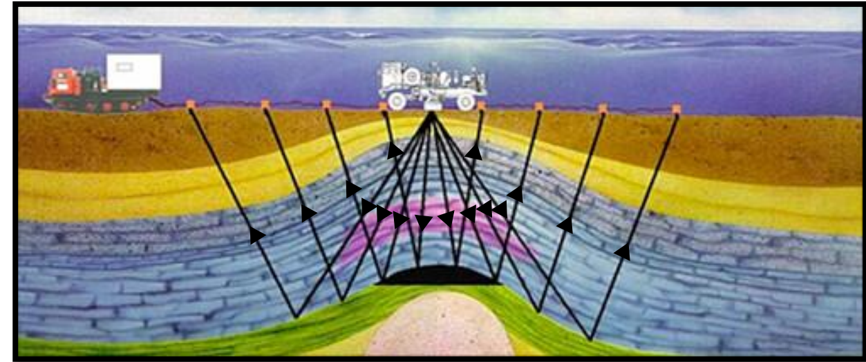
2D Seismic Acquisition showing Vibroseis Truck and geophone receivers – black lines represent path of sound waves from the Vibroseis truck to receivers. The soundwaves travel through each layer of rock at different speeds and this provides an image of the subsurface.
