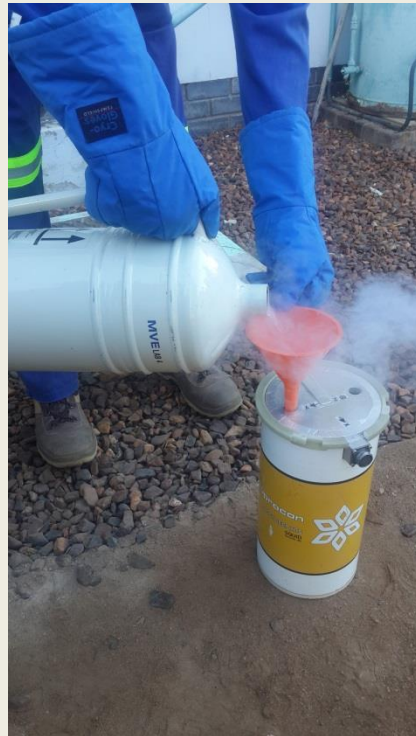
Filling up HT SQUID with liquid Nitrogen
