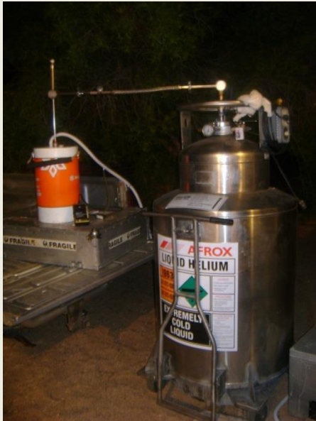
Filling up LT SQUID with liquid Helium
