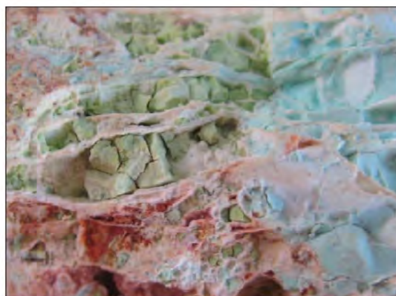
Figure 16. Secondary Ni-rich minerals, Mvurwi section: II. Amorphous, pale green-yellow and pale blue, possible serpentine masses in drusy silica vugs in sheeted silica vein zone. Crude concentrates of this mineral contain > 12.7 % Ni. Width of photograph ca. 3 cm.
