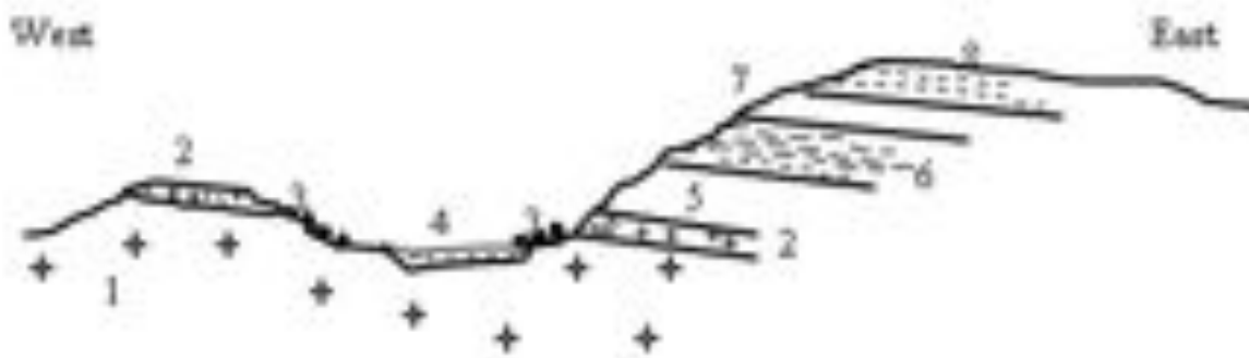
Figure 1. A generalized cross section across the Chiadzwa placer diamond deposit area. 1. Granite basement; 2. Diamond-bearing Umkondo basal conglomerate and arkose; 3. Diamond-rich eluvium shed from the conglomerate; 4. Diamond-rich alluvium; 5. Lower limestone horizon; 6. Lower quartzite horizon; 7. Upper limestone horizon; 8. Upper quartzite horizon.
