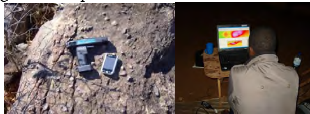
GDD MPP-EM2S+ Magnetic susceptibility and conductivity probe
