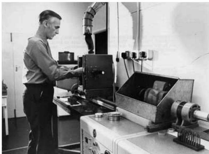
Figure 3: Ian Green with his arc-emission optical spectrograph tended at the ZGS from 1956 to 1986 You had to be careful, and to wonder at the ubiquitous use of the minus 80-mesh fraction of stream sediment and soil samples. That fraction was believed to be most representative of the mix of relatively coarse and fine particles, whether the search was for dispersed copper bonded to the clay fraction, or for nickel in leached and mechanically dispersed fragments of gossan.
